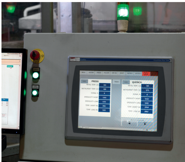
SPOT AL EQS at the press exit and quench displayed on the customer's PLC.
