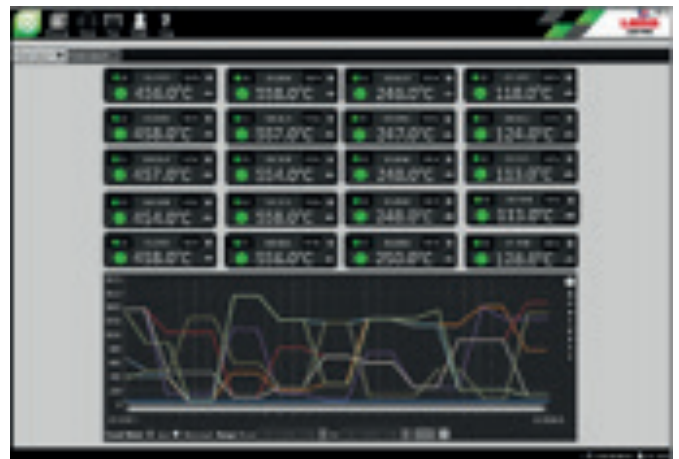
Optional SPOTServe software allows up to 40 SPOT pyrometers to be displayed and data logged.
