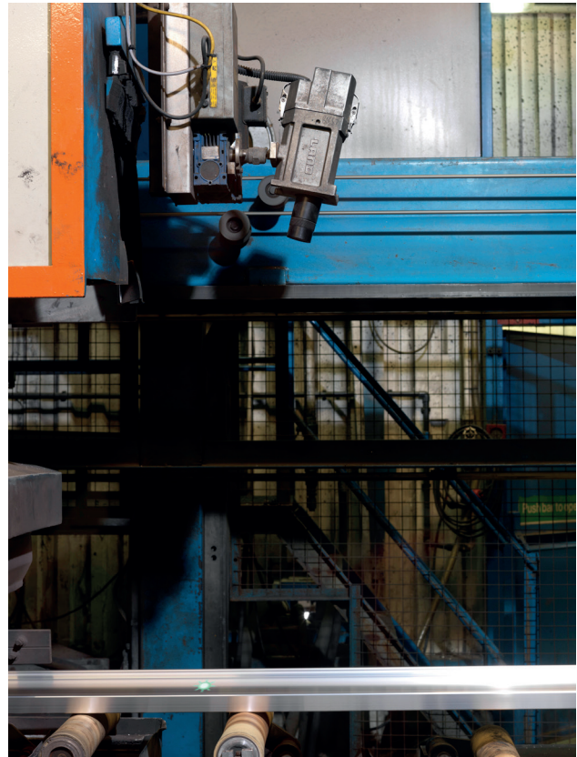
SPOT AL EQS at the quench exit. Green target LED is activated.
