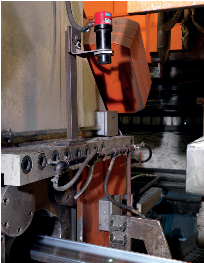
SPOT AL EQS at the press exit. Green target LED is activated.
